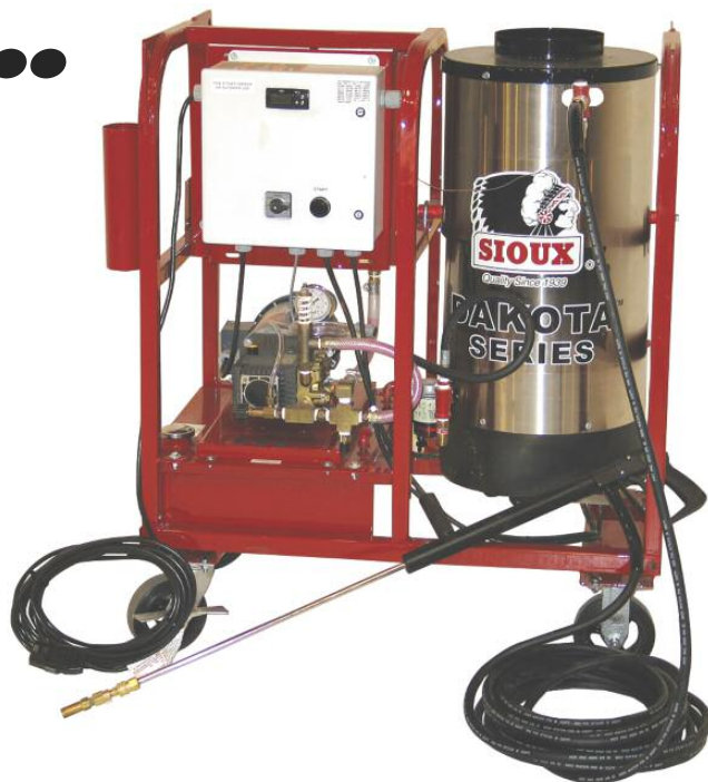
Model S1.5D250 Steam Cleaner 0.75 HP, 1.5 GPM, 250 PSI, Oil Fired
